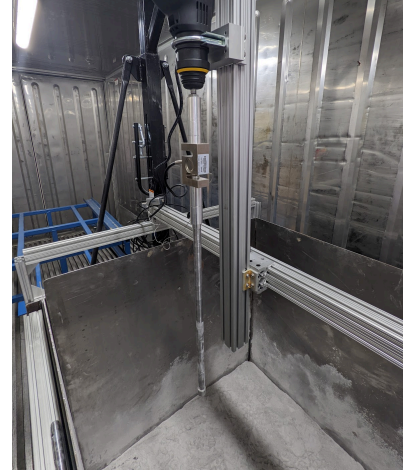
Figure 4: IPCP on a 2D motion stage above a regolith test bin.
